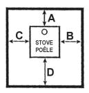
FLOOR PROTECTOR MUST BE NON-COMBUSTIBLE MATERIAL. IT MUST EXTEND BENEATH HEATER, AND TO THE FRONT/SIDEES/REAR AS INDICATED.
